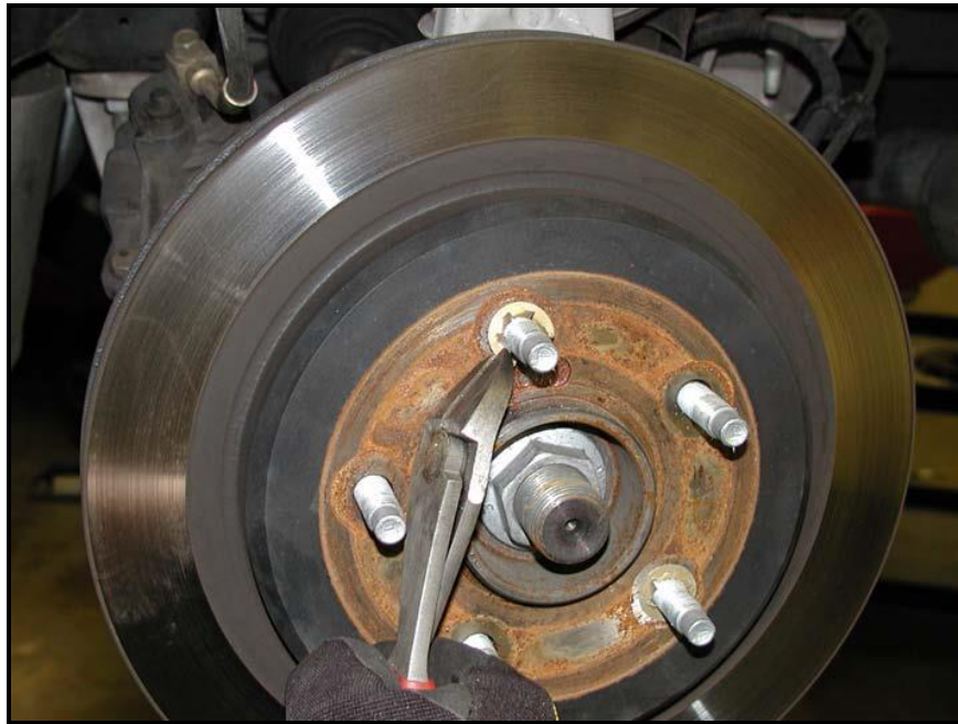
Figure 1: Removal of the Tinnerman nuts prior to rotor removal
