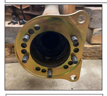
**2.** Install the base steel bracket onto the 5 studs and set in your desired position as shown. The machined side faces outboard. You can clock the bracket for several positions. (Left rear shown) Do not tighten yet.
