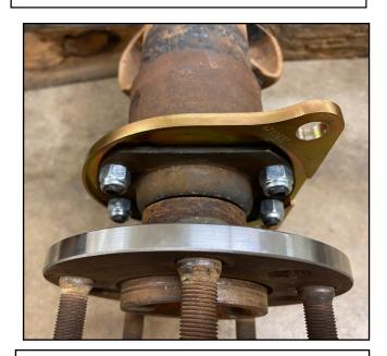
**5**. Secure the 5 studs with your factory nuts. Torque these to the manufacturers spec.
