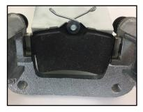
3. Install the pad retention spring into the body of the caliper. From the inside of the caliper body, insert the long tab into the opening and slide it down until the small bent tab clears the piston. Now push the bent tab into the slot and slide it back until it locks onto the ridge on the body as shown.
