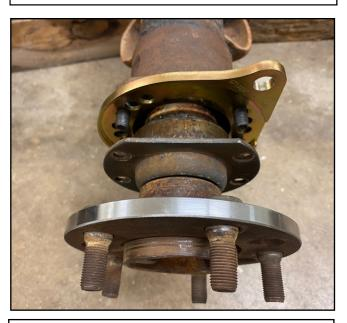
**4.** Next, line up the bearing retainer on top of the Baer bracket and secure with your factory nuts. (**Axle flange diameter not to exceed 6.125**")
