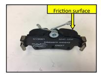
3. Install the pads into the anchor. Put the pad into rotor pathway of the anchor and gently slide the pad and abutments into the inboard side of the anchor. You will be compressing the spring on the side of the abutment as you slide the pad into place. This is a tight fit. Once complete you can do the same for the outboard pad.
