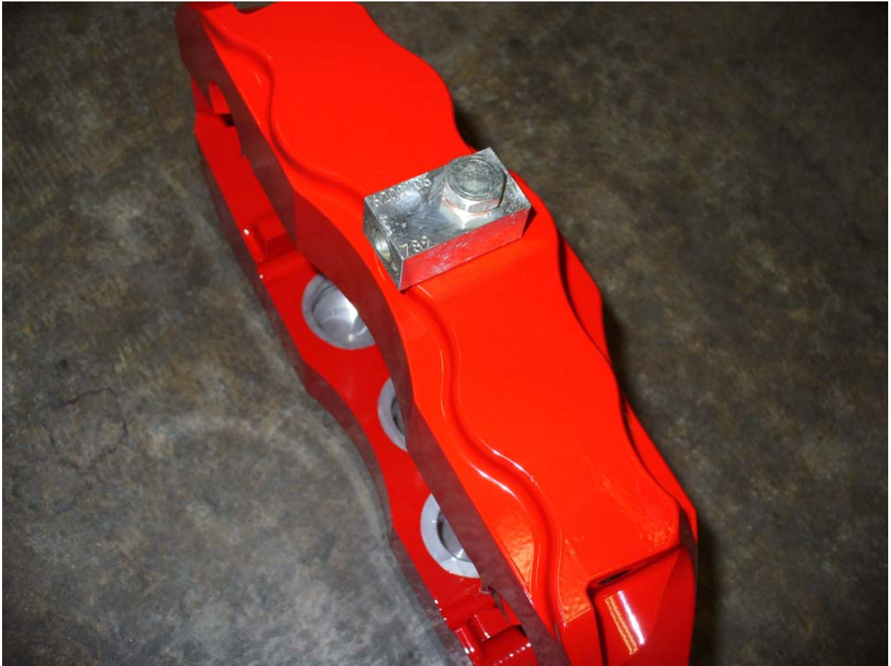
Photo 3: adaptor block installed facing inboard or rearwards-right side shown
