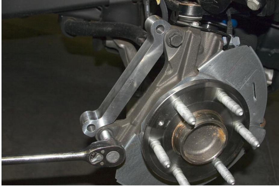
Figure 1 shows the intermediate bracket properly installed. Torque to 110 ft-lbs.
