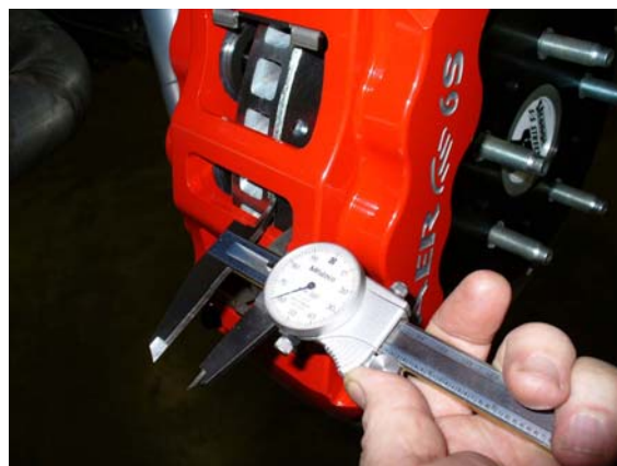
Measure from rotor to caliper body
