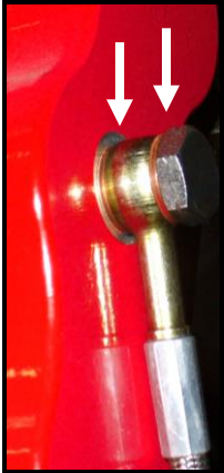
Figure 5: Installation of hose and washers
