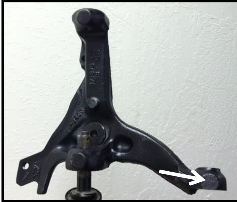
Figure 2: Strike tie rod end boss with large hammer (shown by arrow)
