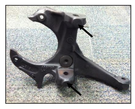
Figure 2: Strike here to dislodge ball joints
