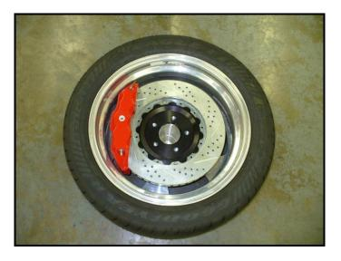
• When installing rotors on any Baer Products be sure to follow the direction of rotation indicated on the rotor hat area with either an arrow, or an "L" for left, or an "R" for right, or both. "L" or left always indicates the driver's side of US spec vehicles. Images shown are "L" left rotors:
