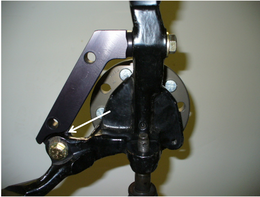
Left spindle with intermediate bracket installed. Arrow indicates shim location if necessary.
