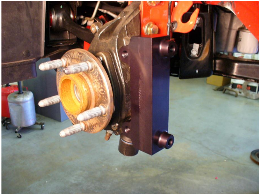
Radial mount installed
