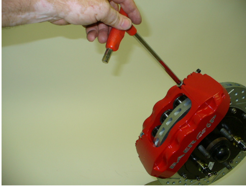
Install the caliper to measure clearance.
