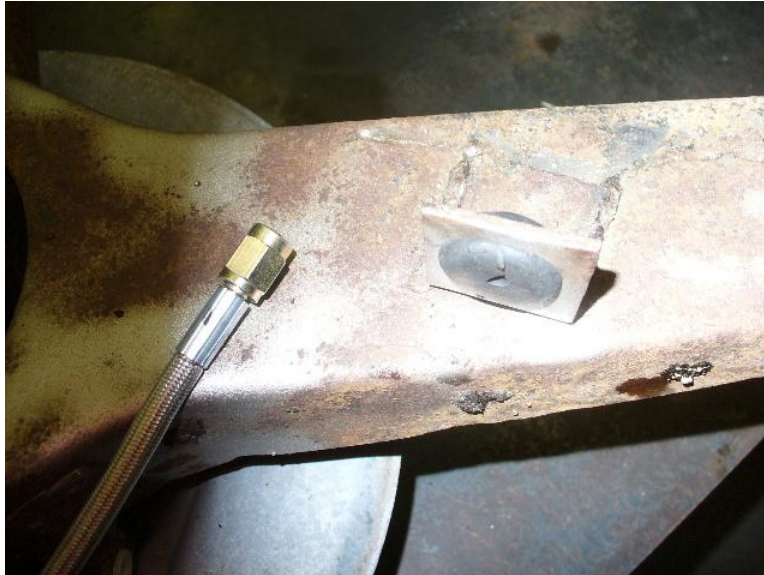
Supplied rubber grommet installed in swing arm bracket
