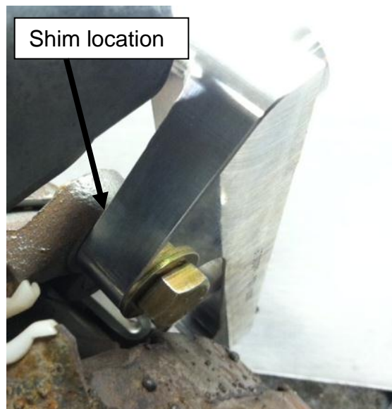
Shim location is between both brackets
