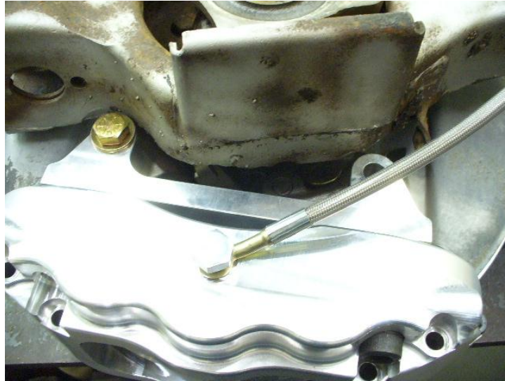
Pro Plus bracket and caliper installed on swing arm
