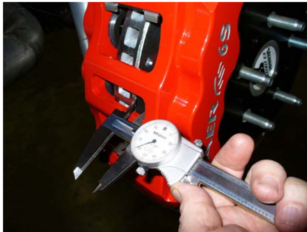
Measuring distance from rotor to caliper body
