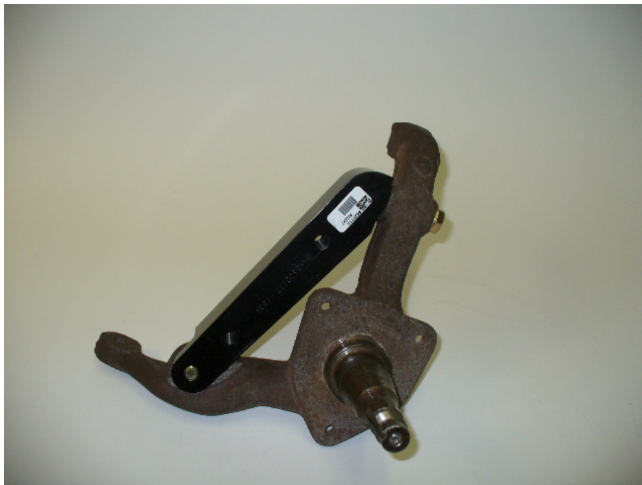
Right spindle with intermediate bracket installed
