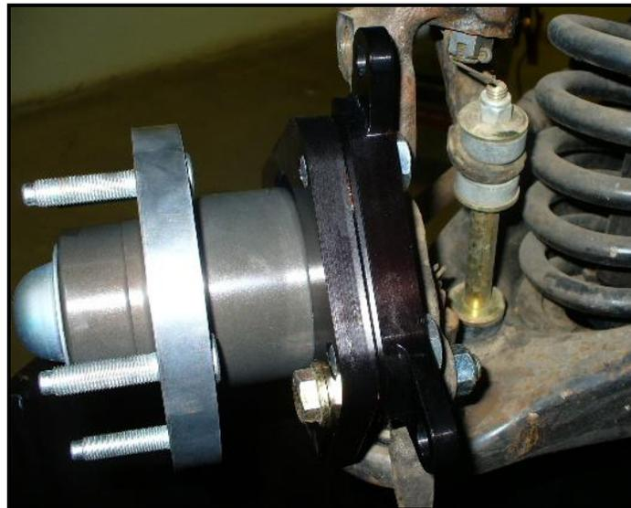
**Intermediate bracket installed
