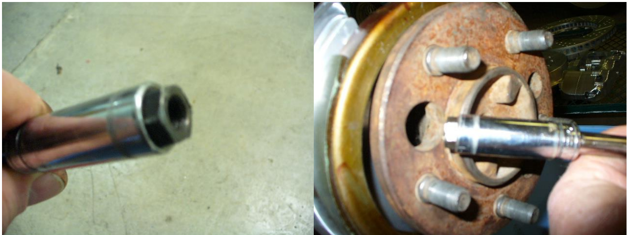
Installing axle retaining nuts
