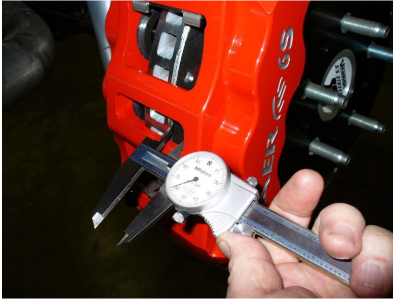
Measuring caliper clearance for centering
