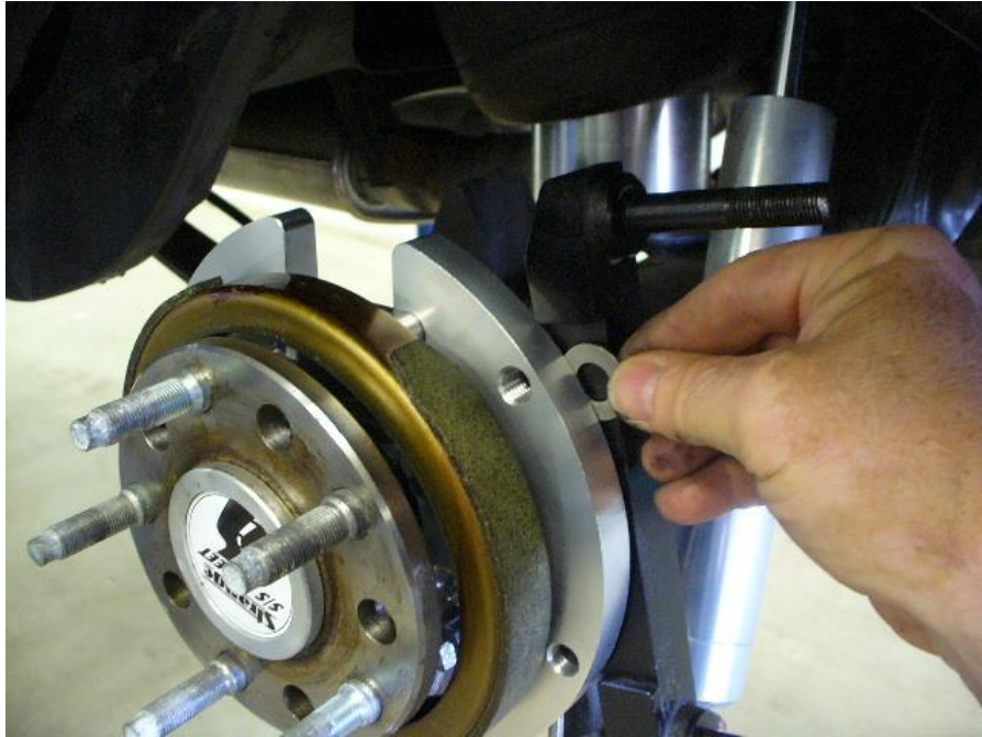
Shims placed between park bracket and radial mount bracket
