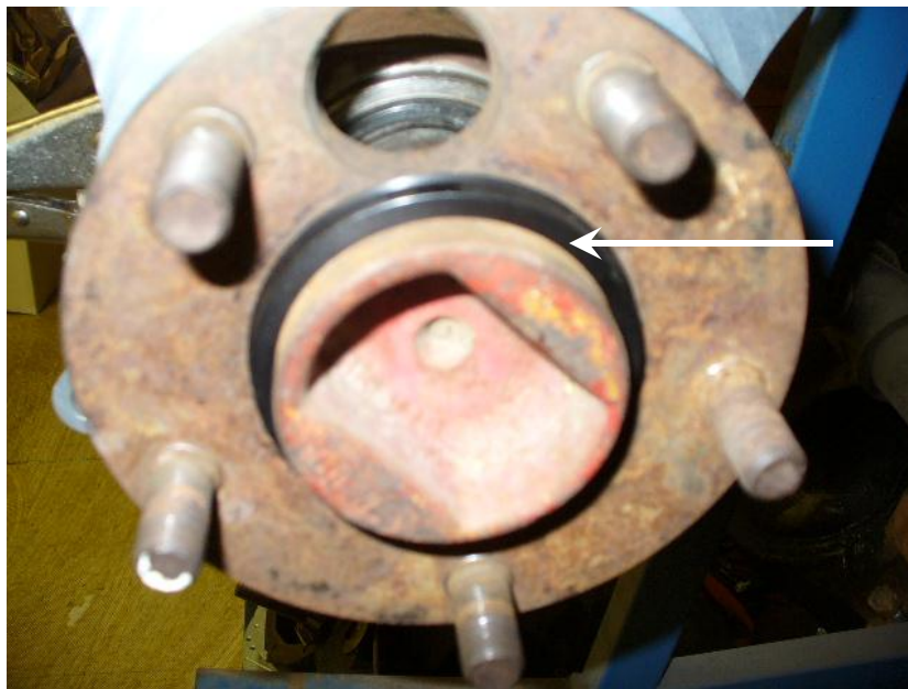
Black centering ring installed over rotor register.
