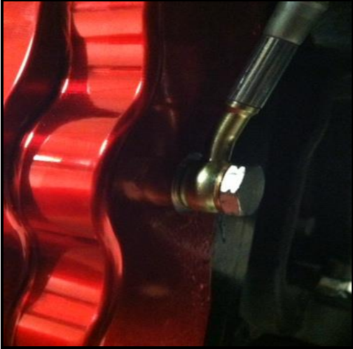
Banjo hose correctly installed
