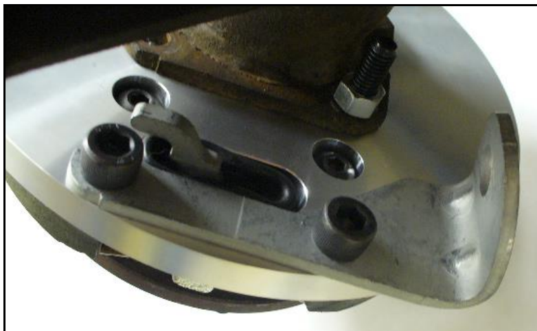
Figure 4: Park assembly installed on driver's side
