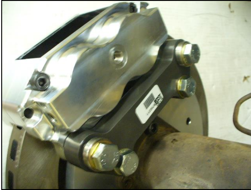
Figure 5: Caliper installed on intermediate bracket.
