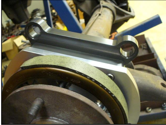
Figure 3: Park brake assembly correctly installed
