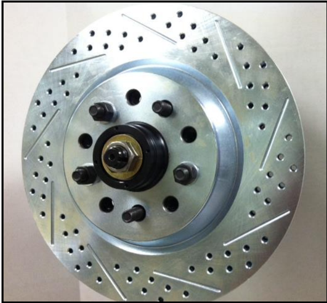
Figure 4: Hub and rotor installed
