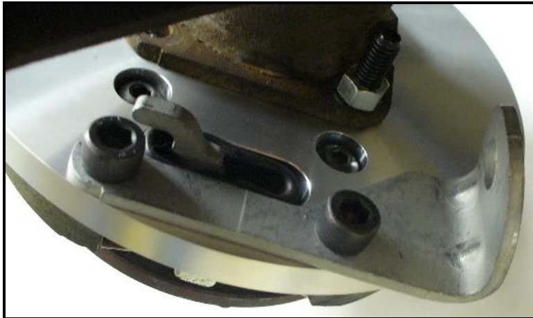
Park assembly installed on driver's side (Actuator is shown at the bottom)
