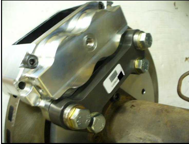
Caliper installed on intermediate bracket.
