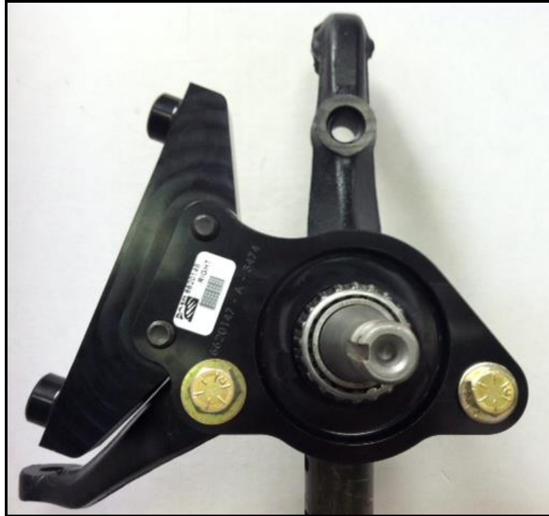
Figure 5: Intermediate bracket installed-Front view
