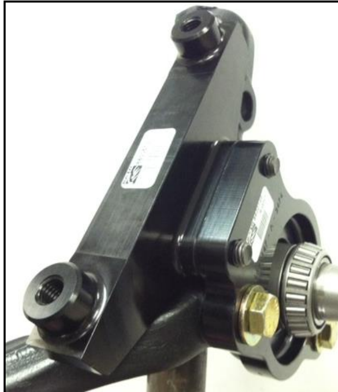
Figure 6: Intermediate bracket installed-3/4 view
