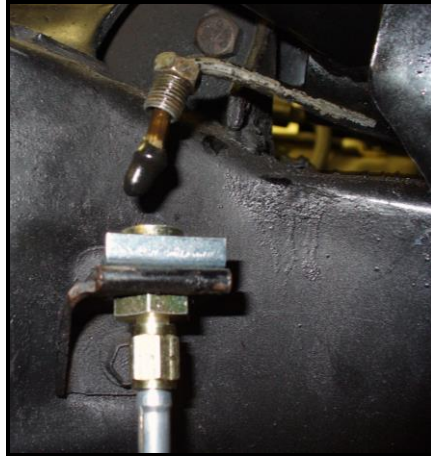
Figure 1: Vinyl cap installed onto hardline
