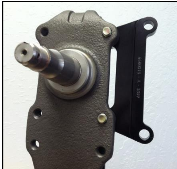
Figure 2: Base bracket installed onto spindle
