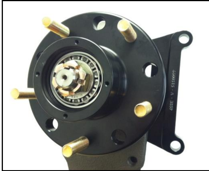
Figure 3: Hub installed onto spindle
