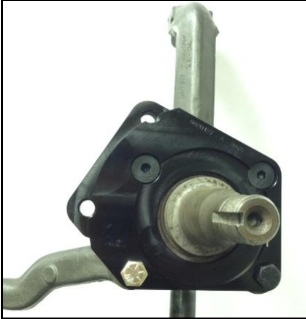
Figure 2: Base bracket mounted to spindle
