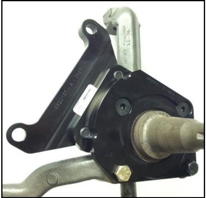
Figure 3: Intermediate bracket bolted to base bracket
