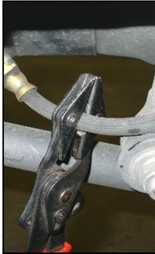
Figure 1: Hose crimper applied to OE brake hose
