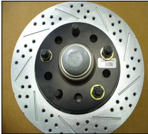
Figure 5: Rotor installed onto hub
