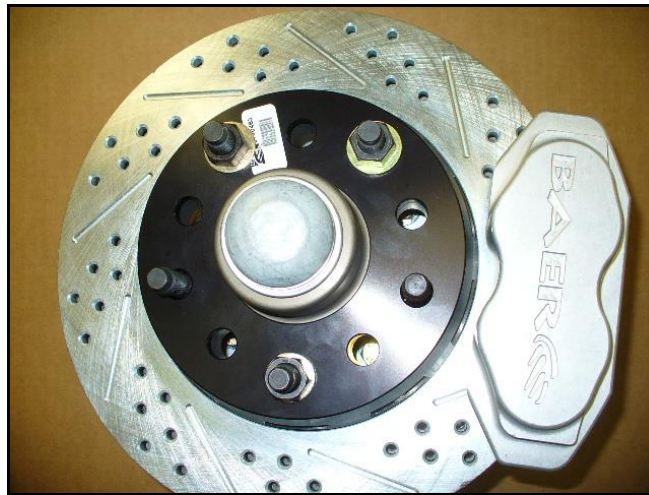
Figure 6: SS4 Caliper installed onto bracket
