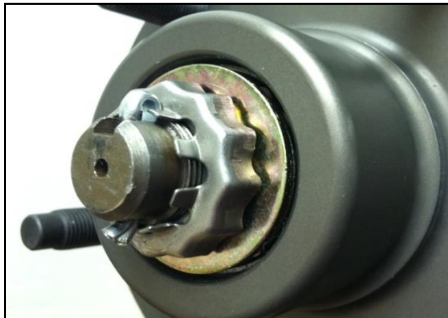
Figure 4: Cotter pin installation
