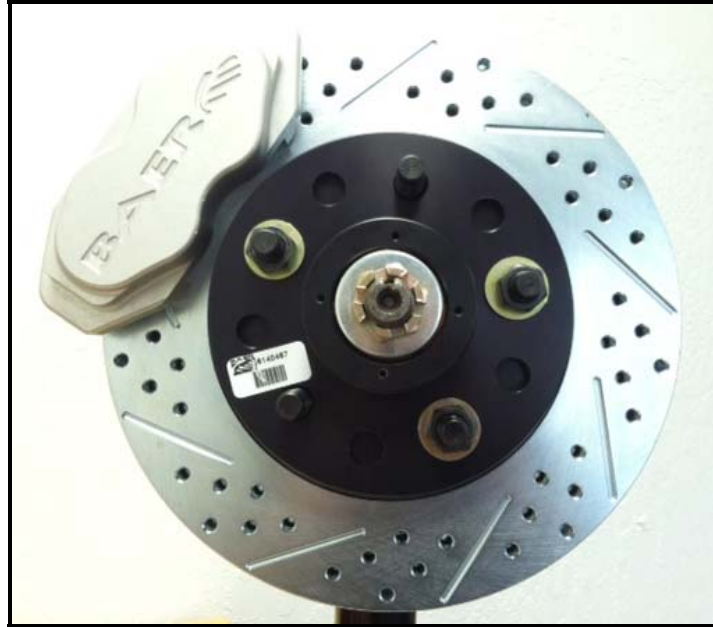
Figure 5: Caliper and rotor installed
