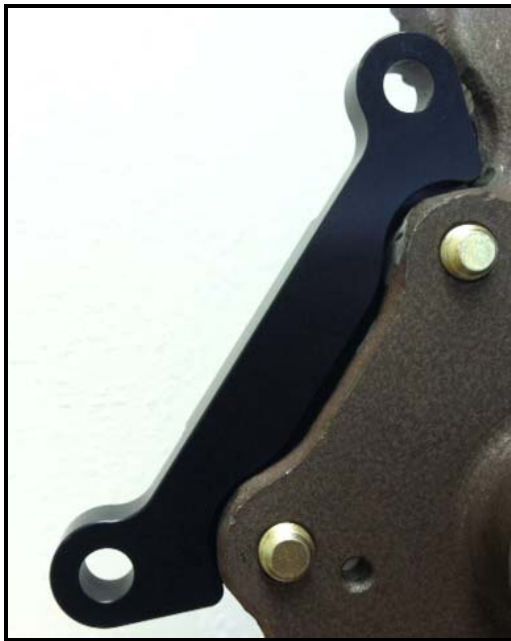
Figure 3: Bracket installed onto passenger side (right) spindle
