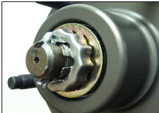
Figure 4: Cotter pin installation
