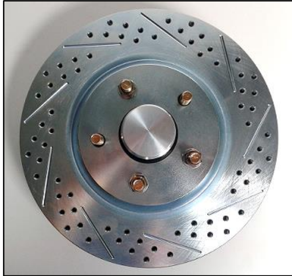
Figure 5: Rotor installed onto hub (drivers side)
