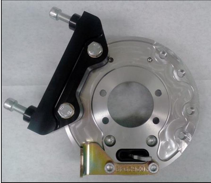
Figure 3: Park brake assembly correctly installed
