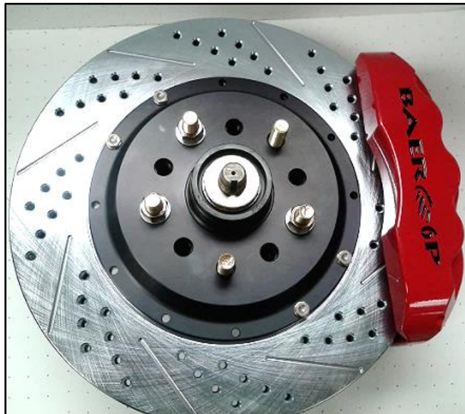
Figure 6: Pro+ caliper installed onto bracket (drivers side)
