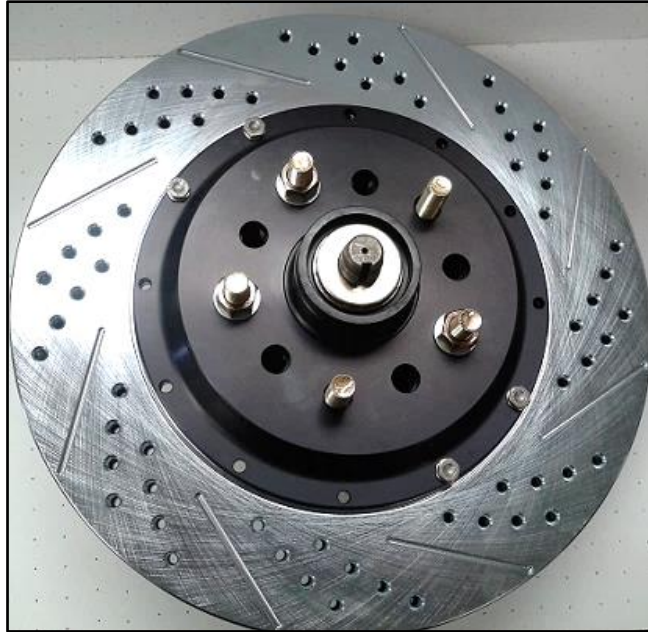
Figure 5: Rotor installed onto hub (drivers side)
