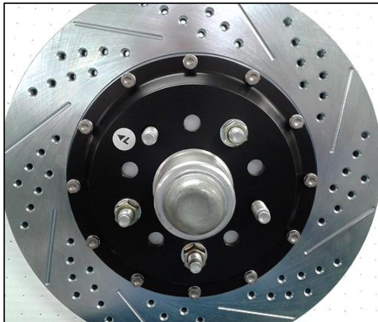
Figure 4: Rotor installed on hub (drivers side)
