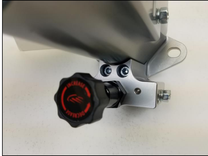
Figure 3: Proportioning Valve Installed to ReMaster
