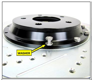
3A . EXTREME +: Thoroughly clean the mating surface of the Hat of any and all corrosion. Place the Hat onto the new Rotor, align the bolt holes and insert the Bolts with Washers as shown.
