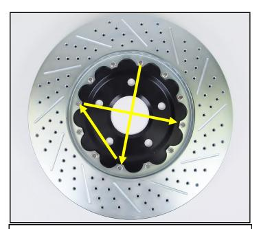
4. Using an in lb torque wrench and a hex socket, torque each Fastener to 180-200 in lbs. or 15-16 ft. lbs. Use an alternating star pattern when torqueing rather than in a continuous series around the perimeter of the Rotor.
