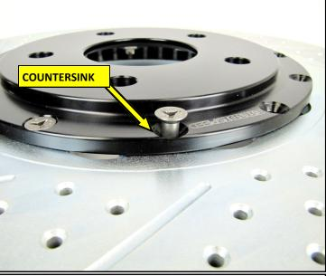
3B. ERADISPEED: Thoroughly clean the mating surface of the Hat of any and all corrosion. Place the Hat onto the new Rotor, align the bolt holes and insert the Tri-Wing Screws into the countersinks as shown.
