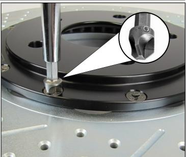
2. ERADISPEED Rotor: Using a 5/16 socket and a #6 Tri-Wing Screw Bit, remove the Screws and nuts securing the Hat to the Rotor Ring. Thoroughly inspect each fastener if they are intended to be reused. NOTE: No other tool can be substituted for the #6 Tri- Wing Bit.
