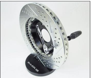
1. EXTREME + Rotor: Using a 5/16 in. socket and 7/16 in. nut driver, remove the Hex Head Bolts, Washers and Nuts securing the Hat to the Rotor Ring. Thoroughly inspect each fastener if they are intended to be reused.
