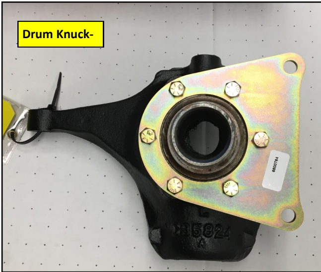
The drum spindle mounts with the steel bracket on top of the spindle.
