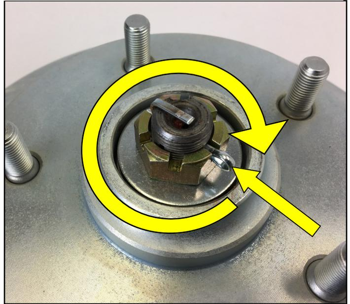
6. Rotate the Rotor to seat the Bearings. Loosen and re-tighten the Nut while spinning the Rotor several times. Tighten the Nut again, to remove any play, approximately 1/16th turn to give a small amount of pre-load. Install the Cotter pin as shown.
