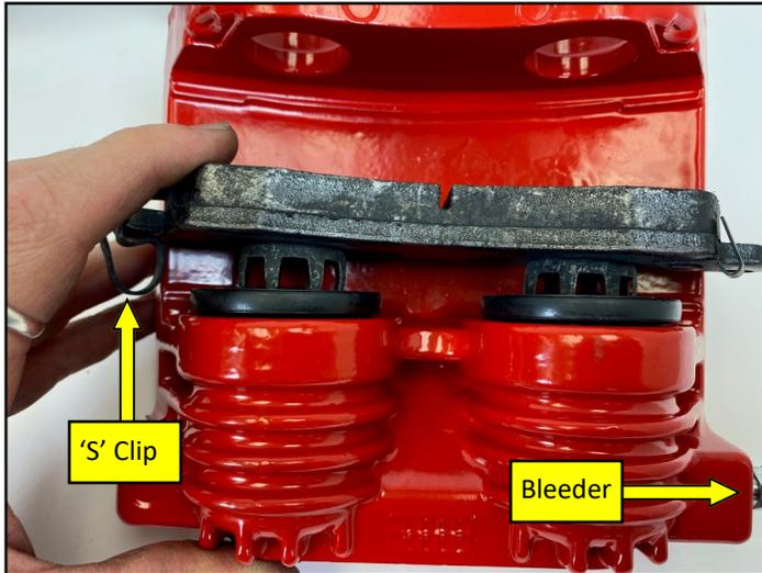
Insert the pad into the pistons as shown. The 'S' clip that you installed should be opposite the bleeder. You may need to bend the star pointers if they are outside the piston holes to get them installed.
