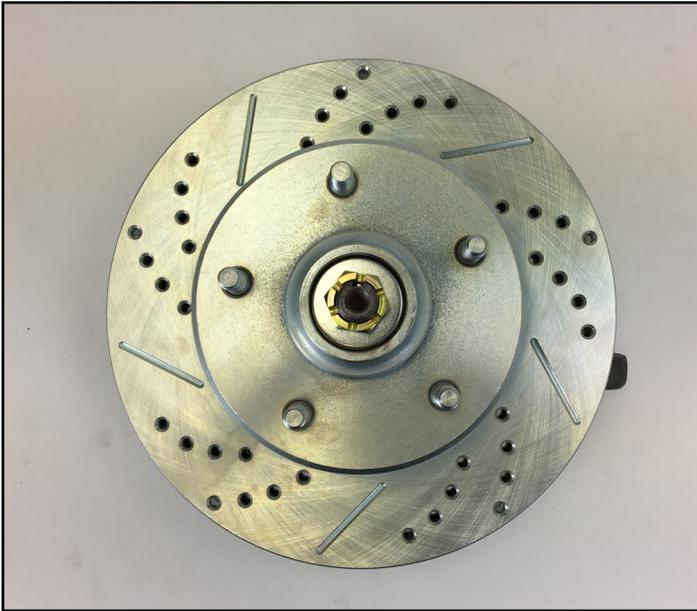
5. Next install the correct side rotor. Thread the spindle nut on and snug. (Right side shown)
