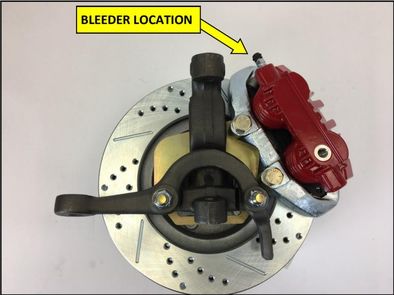
**10.** The caliper should be centered over the rotor. Check for any clearance issues between the anchor and the rotor. If everything is good here, torque the 1/2-13 hex bolts to 105ft-lbs.
