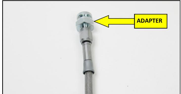
9. Install the new Brake Hose, onto the Caliper with one Crush washer on each side of the banjo fitting. Finger tighten the Banjo Bolt. **IMPORTANT:** Position the hose to avoid interference with the wheel and suspension components. Tighten fitting and banjo bolt to 15-20 ft-lbs.
