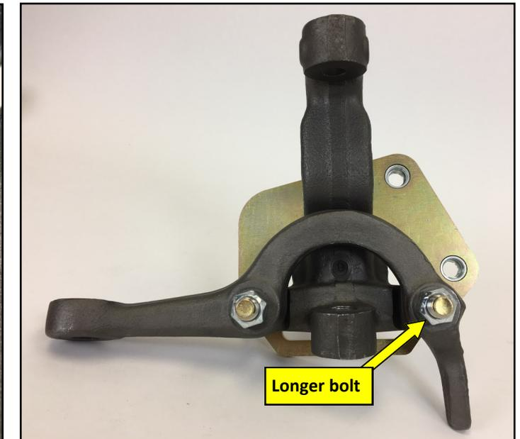
4. Inboard view of the bracket installed. Make sure the PEM nuts are facing outboard and that you used the correct length bolts to ensure threads protrude through the locking stover
