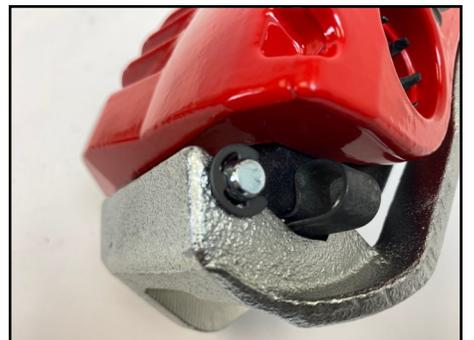
Install the pin from the backside of the caliper into the groove on the anchor. (Where the 'S' clips are) The pin should go all the way through to the front of the caliper. Install the 'E' clip onto the groove on the end of the pin to secure the anchor to the pads. Repeat this process for the other caliper. Now you are ready to install the caliper onto the rotor.
