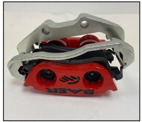
Once the pads are installed you will install the anchor by 'hooking' the curved inside notch around the pads and pushing it down into the 'S' clips. Push the anchor past the 'S' clips until they are inside the anchor.
