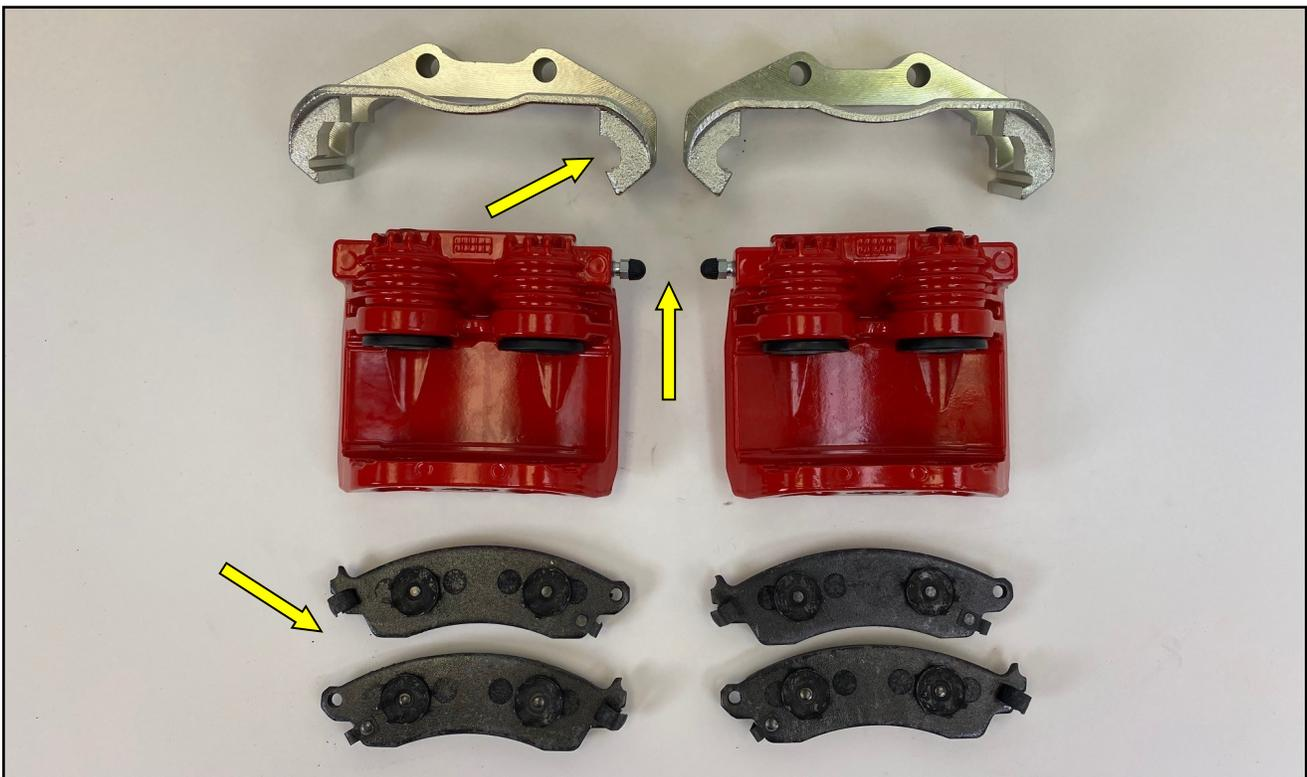
Lay out the calipers, anchors and pads as shown. This means the right caliper and anchor are on the right and left caliper and anchor is on the left. And one of each pad per caliper.
