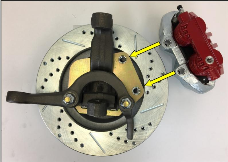
**9.** Now install the correct side caliper with the bleeder pointing up. Use the supplied 1/2-13 hex bolts and washers and hand tighten for now.
