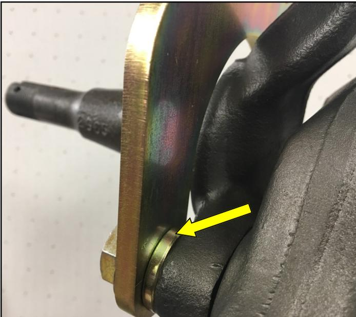
3. The .150" spacers go between the bracket and the spindle.
