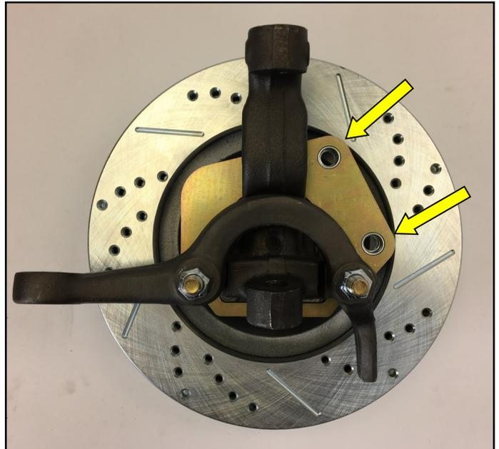
8. Inboard view of rotor installed. Check these areas for any clearance issues between the bracket and the rotor. There can be casting variances on the rotor. If needed, grind the bracket MINIMALLY to clearance.
