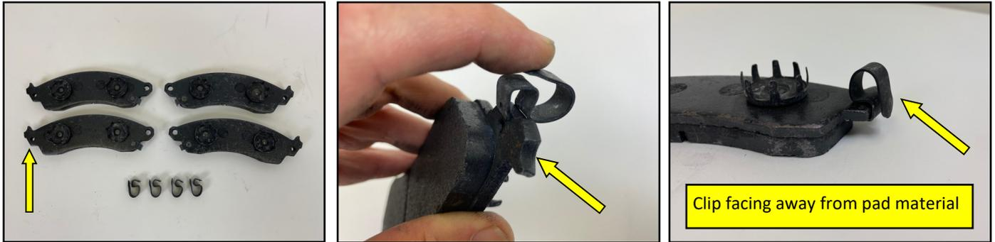
Install the supplied 'S' clips onto each pad. The clip goes on the side of the pad with the notch for the pin. Make sure the clip is facing away from the pad material.
