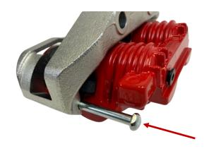
INSTALL THE PIN FROM THE BACKSIDE OF THE CALIPER INTO THE GROOVE BETWEEN THE ANCHOR AND PADS, WHERE THE 'S' CLIPS ARE.
