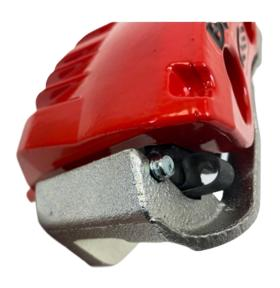
PUSH THE PIN THROUGH THE OUTSIDE GROOVE BETWEEN THE ANCHOR AND PAD.
