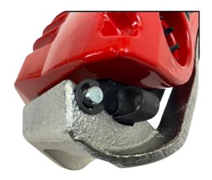
INSTALL THE E-CLIP INTO THE GROOVE ON THE END OF THE PIN STICKING THROUGH
