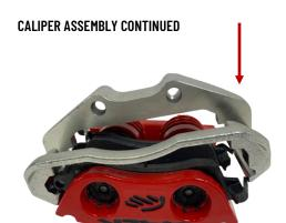
PRESS THE ANCHOR DOWN INTO THE 'S' CLIPS INSTALLED IN THE CALIPER. YOU MAY HAVE TO COMPRESS THE 'S' CLIPS TO PRESS THE ANCHOR DOWN.
