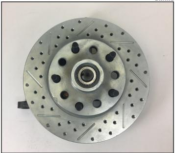
**5.** Next install the correct side rotor. Be careful not to damage the wheel seal when going over the base of the spindle pin. Thread the spindle nut on and snug. (Right side/passenger shown)
