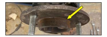
**4.** Next install the axle back into the housing. Re-install the cclips, axle retention pin and screw. Baer recommends not installing the rear diff cover and fluid until you have verified both sides are complete and that you will not need to remove the axles again. Clean off the axle rotor register and make sure it is free from rust and debris. This will ensure the rotor is sitting flat against the axle flange.
