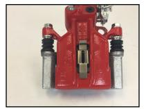
2. Install each pad abutment onto the 'ears' of the caliper. The abutment should face away from the friction surface. There is a small tab that locks into place once installed correctly.
