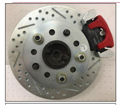
**9.** View of caliper and rotor installed. Drivers side shown. (Left side). Install the hose to the caliper using the supplied banjo bolt and crush washers. Use 1 crush washer on each side of the banjo bolt. Make sure the hose doesn't interfere with any suspension components or the tire/wheel. Torque the banjo bolt to 15 ft lbs.
