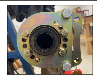
**2.** Bolt the steel intermediate bracket to the inboard side of the base bracket using the supplied 12mm bolts, washers, spacers and lock nuts. Torque the bolts/nuts to 85ft lbs.
