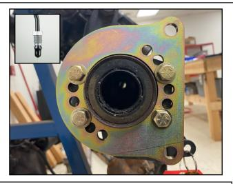
1. Install the base steel bracket using the factory bolts in your desired position using the factory hardware. You can clock the bracket in several positions. Check for any clearance issues with suspension components. (Driver side/Left rear shown) Torque the factory bolts to the manufacturers specs.
