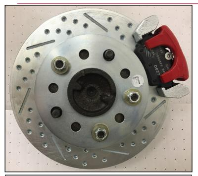
**8.** View of caliper and rotor installed. Driver side shown. (Left side). Install the hose to the caliper using the supplied banjo bolt and crush washers. Use 1 crush washer on each side of the banjo bolt. Make sure the hose doesn't interfere with any suspension components or the tire/wheel. Torque the banjo bolt to 15 ft lbs.
