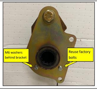
2. Install the Bracket onto the outboard side of the rear end housing. Put a single M6 washer between the bracket and rear end of the 2 lower bolts. This will allow the bracket to sit flat against the rear end. You will reuse your factory bolts for the 2 lower holes. Torque these to the manufacturers spec.
