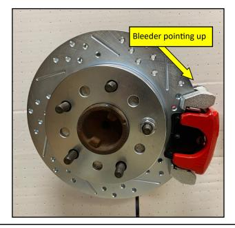
**7.** Install the correct side caliper making sure the bleeder is pointing up.
