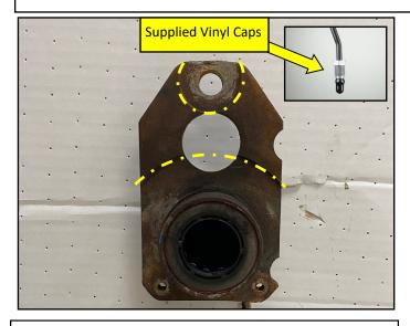
1. This installation begins at the point at which the OE brake components and axles have been removed from the vehicle and the hard lines have been capped with the provided vinyl caps to prevent fluid leak down. (Driver Side Shown) Because the rear end flange is not flat, you will be putting shims behind the steel bracket.
