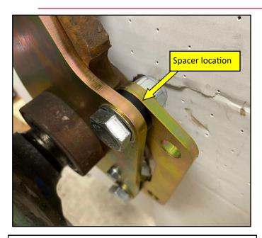
**5.** Next install the intermediate bracket to the inboard side of the base bracket. Use the supplied 12mm hex bolts, washers, spacers and nylock nuts. The spacer goes in between the base bracket and the intermediate bracket. **Torque these nuts to 85ft lbs.**
