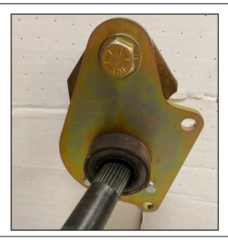
**4.** Install the axle back into the rear end and install the clip and rear end pin. Repeat this process for the passenger side. **DO NOT** finish the rear end until you have verified the install is complete.
