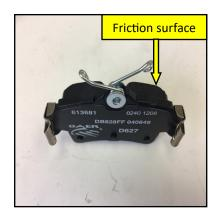
3. Install the pads into the anchor. Put the pad into rotor pathway of the anchor and gently slide the pad and abutments into the inboard side of the anchor. You will be compressing the spring on the side of the abutment as you slide the pad into place. This is a tight fit. Once complete you can do the same for the outboard pad.
