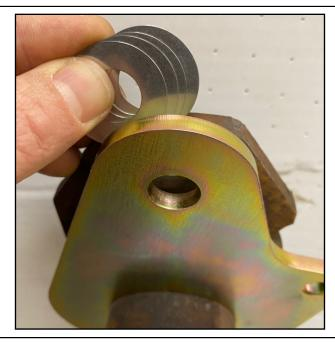
**3.** Put (4) of the supplied 5/8" shims between the top of the bracket and the top of the rear end. This will allow the bracket to sit flat against the rear end. Install the supplied 5/8" hex bolt and nut. **Torque this nut to 145ft lbs.**
