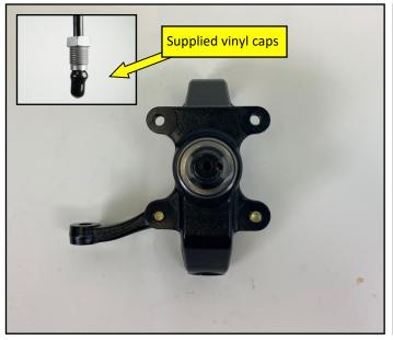
**1.** This installation begins at the point at which the existing brake components have been removed and the hard lines have been capped to prevent leak down. (Driver side/Left side shown)
