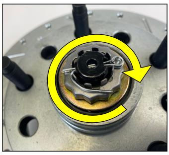
**6.** Next install the spindle nut. Tighten the nut to seat the Bearings. Loosen and re-tighten the Nut while spinning the Rotor several times. Tighten the Nut again, to remove any play, approx. 1/16th turn to give a small amount of pre-load. Finally install the retainer & cotter pin. Cut & bend.
