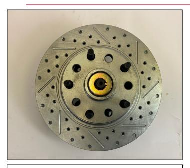
**5.** Install the correct side rotor (Driver side shown). Be careful not to damage the wheel seal when going over the base of the spindle pin.
