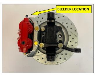
10. The caliper should be centered over the rotor. Check for any clearance issues between the anchor and the rotor. If everything is good here, torque the 1/2 hex bolts to 110ft lbs. If there are any clearance issues or your caliper is not centered over the rotor, remove the caliper/rotor and double check that the bracket is flat against the spindle and that the rotors bearings are completely seated against the spindle pin.
