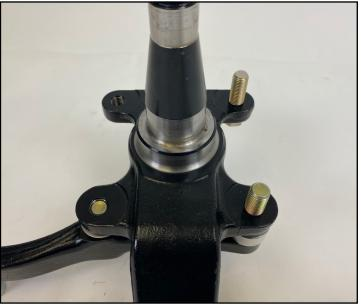
**2.** Start by threading the supplied 7/16" hex bolts & washers all the way from the inboard side through the spindle as shown. The lower bolt is longer and will go through the steering arm and spacers that came with your spindle.
