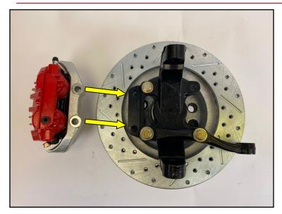
**9.** Now install the correct side caliper with the bleeder pointing up. Use the supplied 1/2" hex bolts and washers and hand tighten for now.
