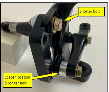
**4.** Inboard view of the bracket installed. The shorter bolt goes at the top and the longer bolt goes through the steering arm & spacers at the bottom.
