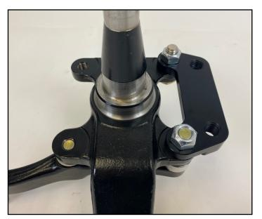
**3.** Slide the bracket onto the bolts as shown and secure with the supplied 7/16" stover nuts. **Torque these nuts to 75ft lbs**.
