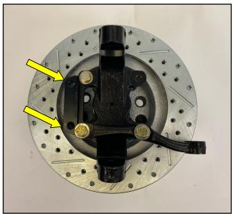
**8.** Inboard view of rotor installed. Check these areas for any clearance issues between the bracket and the rotor.
