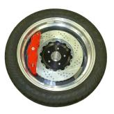
• When installing new Baer rotors, be sure to follow the direction of rotation indicated on the rotor hat area with either an arrow, or an "L" for left, or an "R" for right, or both. "L" or left always indicates the driver's side of US spec vehicles. Images shown are "L" left rotors:
