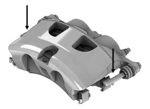
APPLY A <u>Small amount</u> of caliper Pin Grease to Each of the sliding Pins on the caliper. (Brake Hose not shown in Photo, disconnection of origi-Nal Brake Hose Not Required)
