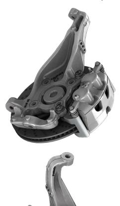
INSTALL THE CALIPER ASSEMBLY WITH THE NEW BAER ERADISPEED F -150 ANCHOR TO THE OUTBOARD SIDE OF THE MOUNTING EARS ON THE KNUCKLE, SAME AS THE ORIGINAL. USE THE ORIGINAL FASTENERS TO SECURE THE CALIPER ASSEMBLY TO THE KNUCKLE. TORQUE THE FAS-TENERS TO 136 FT-LBS. TO SECURE THE CALIPER ASSEMBLY TO THE KNUCKLE. (BRAKE HOSE NOT SHOWN IN PHOTO, DISCONNECTION OF ORIGINAL BRAKE HOSE NOT REQUIRED)
