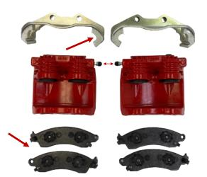
LAY OUT THE CALIPERS, ANCHORS, AND PADS AS SHOWN. THE RIGHT CALIPER AND ANCHOR ARE ON THE RIGHT AND THE LEFT CALIPER AND ANCHOR ARE ON THE LEFT. THE BLEEDER SCREWS SHOULD FACE EACH OTHER. THE CURVED NOTCH IN THE ANCHORS SHOULD FACE EACHOTHER. THE PADS SHOULD BE LAID OUT WITH ONE OF EACH SIDE.
