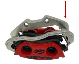
PRESS THE ANCHOR DOWN INTO THE 'S' CLIPS INSTALLED IN THE CALIPER. YOU MAY HAVE TO COMPRESS THE 'S' CLIPS TO PRESS THE ANCHOR DOWN.
