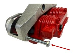
INSTALL THE PIN FROM THE BACKSIDE OF THE CALIPER INTO THE GROOVE BETWEEN THE ANCHOR AND PADS, WHERE THE 'S' CLIPS ARE.
