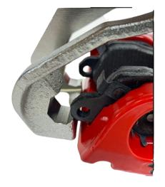
HOOK THE CURVED INSIDE NOTCH ON THE ANCHOR AROUND THE PADS AS SHOWN. (PADS MAY OR MAY NOT HAVE WEAR INDICATORS ON BOTH INSIDE AND OUTSIDE PAD)
