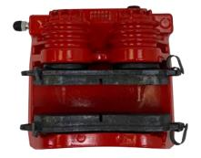
LAY THE CALIPER WITH THE CORRESPONDING ANCHOR AS SHOWN. (PADS MAY OR MAY NOT HAVE WEAR INDICATORS ON BOTH INSIDE AND OUTSIDE PAD)
