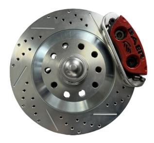
11. Install the correct side caliper to the previously installed base bracket with the bleeder screw pointing up. Secure the caliper to the base bracket with the supplied M12-1.75 x 30mm bolts and washers. Thread locker is not necessary. Torque the supplied hardware to 85 ft-lbs. to secure the caliper to the base bracket.
