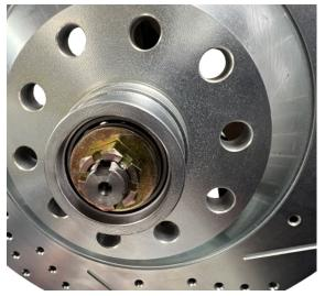
5. Install the provided castle nut as shown. Rotate the rotor while tightening the castle nut to seat the bearings. Loosen and retighten the nut while spinning the rotor several times. Tighten the nuts again to remove any end play, approximately 1/16th of a turn to give a small amount of pre-load.
