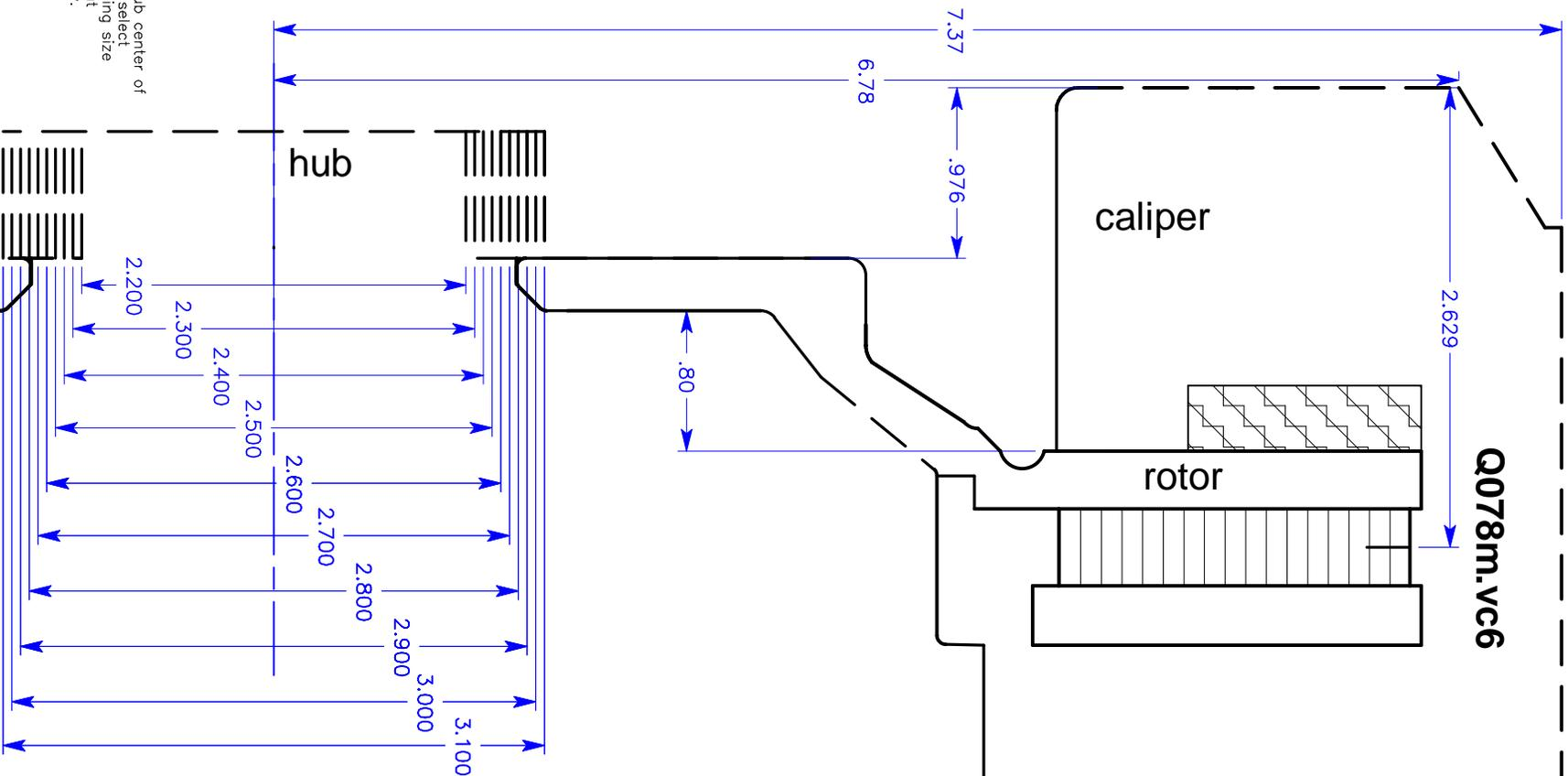
Measure hub center of the wheel, select corresponding size and cut out accordingly.
